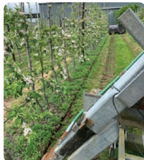
Figure 4. AMF were inoculated on tree roots using a modified root pruner with an attached stocks applicator, developed by Agrovista
